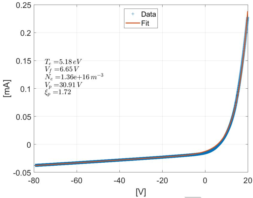
**FIGURE 4.** Example of a Langmuir probe IV curve recently obtained with custom-made diagnostic circuits.
