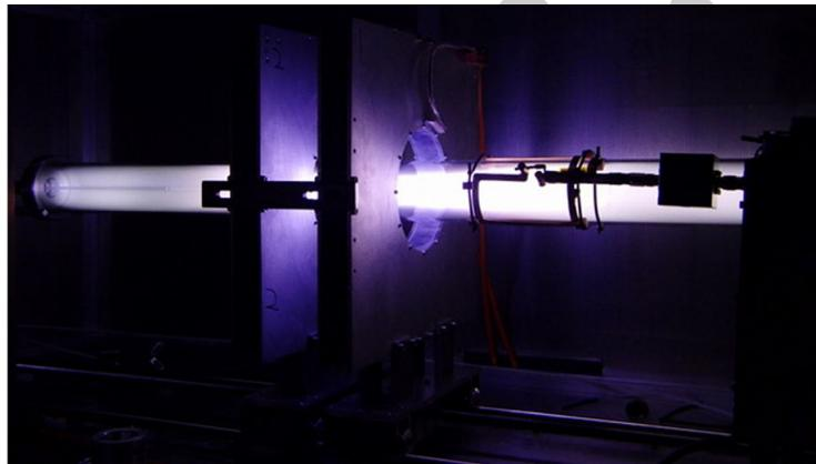
**FIGURE 6.** A RF plasma discharge into the SP3 Echidna experiment. Adapted from [13].
