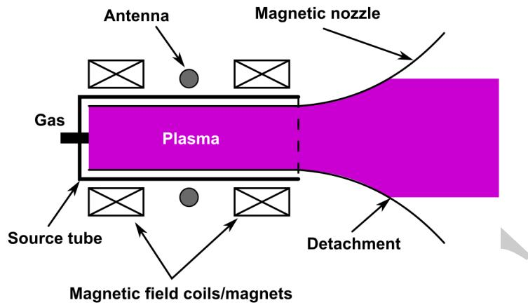
**FIGURE 5.** Cartoon of a Helicon Plasma Thruster with its various components. Adapted from [12].
