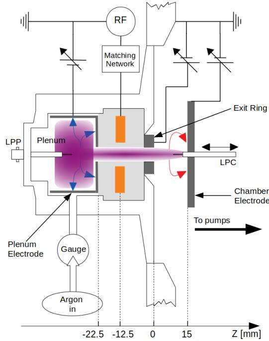
**FIGURE 2.** Sketch of the ePR, with a set of collecting electrodes allowing it to operate as a neutraliser.
