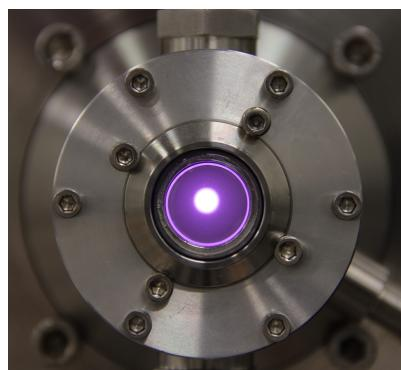
**FIGURE 1.** Argon discharge in ePR, as viewed through the plenum window.
